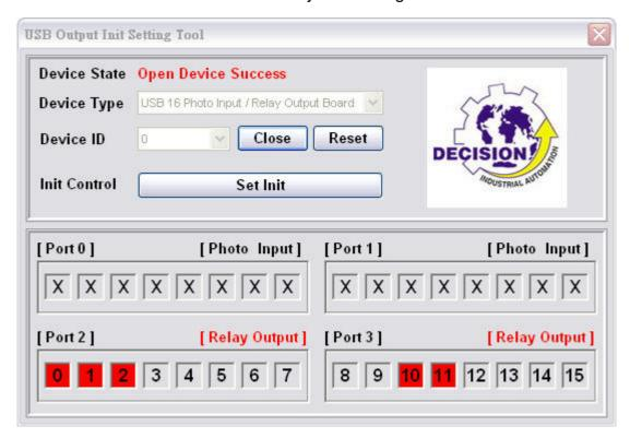
5. When finishing setting, please press the reset button on the board. And please use this tool carefully due to init value you set will be loaded when power on, it may cause damage for its init state changed.
