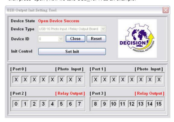
**4.** You can set init value on output port by clicking the output bit and press "Set Init" when finished. It should show synchronizing on the board.
